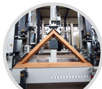
Spitzfensterausrüstung Accessory kit for pointed frames
